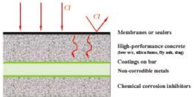
Fig. 4: There are multiple methods available to protect concrete from corrosion damage.
