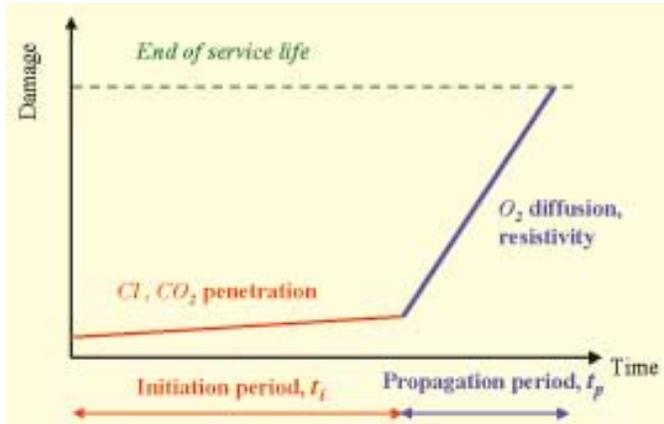
Fig. 3: Life-365 estimates the time it takes for a structure to reach the end of its service life. The initiation period  $t_i$  is the time it takes for chlorides to penetrate the concrete cover and accumulate at the reinforcement. The propagation period  $t_p$  is the time it takes for corrosion to reach an unacceptable level.
