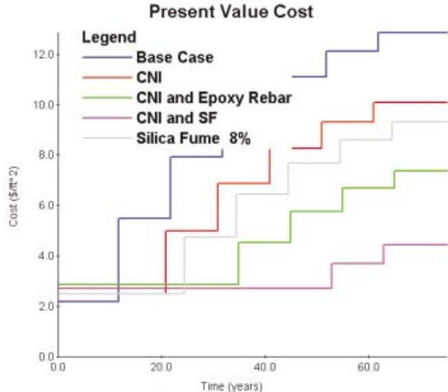
Fig. 7: Total life-cycle costs as the sum of initial construction costs and discounted future repair costs over the life of the structure for several corrosion-protection methods
